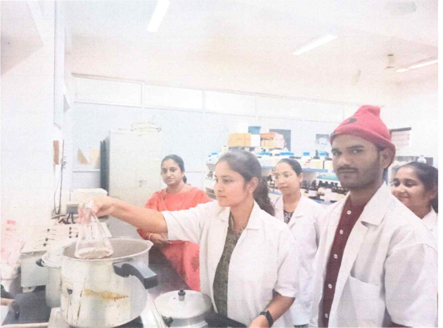
Department of Genetics & Genomics – Mini Autoclave for sterilization of Media
